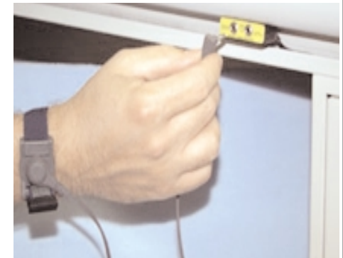
Use a dual wire constant monitor with dual wire wrist straps.
